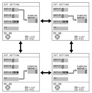
The arrow in the menu represents a signal flow. The left side of the arrow shows a signal source output from the EXT-2 terminal.
