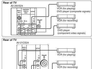
When you use VIDEO-1 INPUT, you should choose to connect S-VIDEO or video input. If S-VIDEO connector and video input are connected at the same time, no picture displays on the screen and the message "PLEASE DISCONNECT VIDEO-1 CABLE!" appears. In this case, you should disconnect either S-VIDEO or video input.
