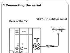
If you connect a VCR, connect the aerial output jack of your VCR and the aerial jack on the TV with the aerial cable. Then connect the output jacks of your VCR and the VIDEO-1 input jacks of the TV with the video cable and audio cables. For details, see the manual of your VCR.
