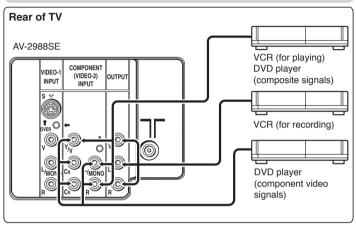
When connecting to COMPONENT (VIDEO-2) input, depending on the connection, choose the appropriate video input using the menu (see "VIDEO-2 SETTING" on page 18)
