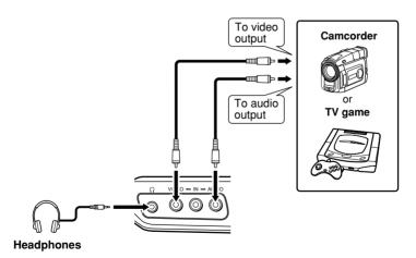
• Use the headphones with a stereo mini jack (3.5 mm in diameter). When you connect the headphones, the TV speakers go off.
