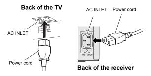
Insert the AC plug into a correctly earthed outlet.
