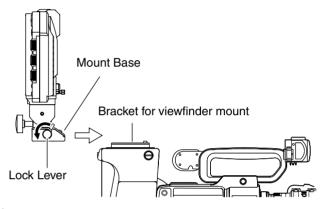
3 Rotate the viewfinder lock lever as shown in the direction of the arrow ( → ) and secure the viewfinder to KA-HD250U.
