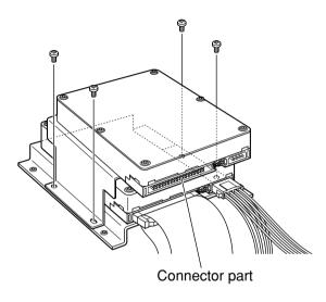
**4.** Connect the hard disk power cable and flat cable to the connectors on the SA-K51U.
