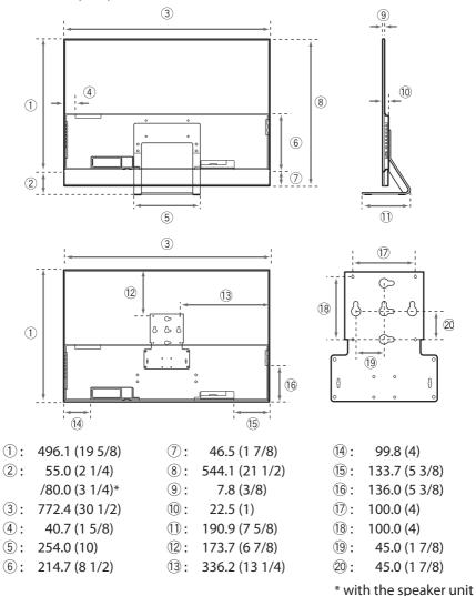
$\bullet$  Use screws of adequate length (M4  $\times$  12 – 16) to fix the VESA bracket and wall mount adapter.
