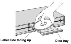
Place the disc on the disc tray with the label side facing up. Since disc size changes depending on the disc to be played back, be sure to correctly align the disc with the grooves for its size. If the disc is not in its groove, it may be scratched or otherwise damaged. To insert an 8 cm disc, place it according to the inner groove.
