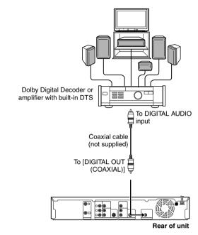
1 Connect the unit and a Dolby Digital Decoder or an amplifier with built-in DTS using an optional coaxial cable.
