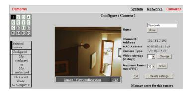
On the left side of the screen, a 4x4 matrix is available that allows the administrator to easily switch between any of the 16 cameras from within this same window. This is standard when viewing details for all camera types.
