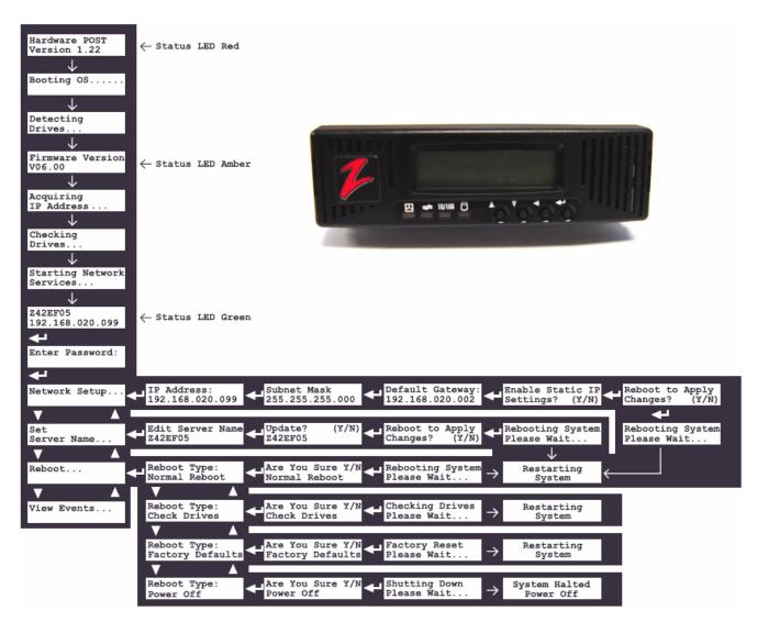
Each key has a different function, illustrated by a directional arrow just above and to the left of the key.
