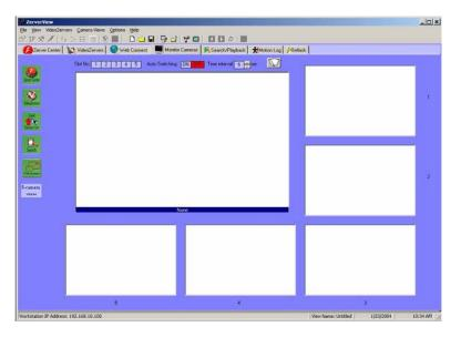
4. On the left side of the page, click on Load Camera List button to open the Camera List dialog box. From within this window, you only need to drag-and-drop the cameras which you want to use for this view into the corresponding blank camera window so that VDRView can link that camera into the view. Cameras can be from the same or different VR-N100Us. Once you are done, you can close the dialog box.
