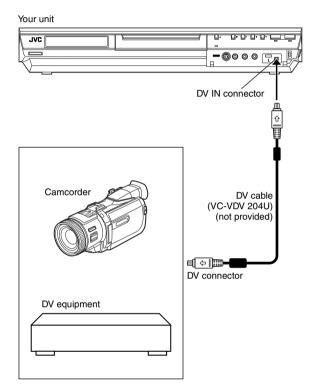
1 Connect a camcorder or DV equipment to the DV IN connector on the unit's front panel.
