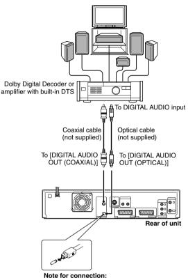
Remove the protection cap from the optical cable.
