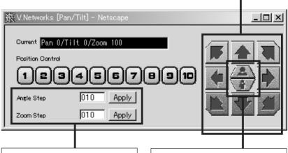
The current [Zoom Step] and [Angle Step] settings for the pan/tilt operation are displayed.
