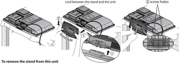
Unscrew the screws indicated by above "(3)". screw holes. After the screws are removed pull the stand up toward the rear of the unit. Be careful not to drop the stand when you remove it.
