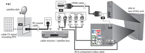
You can also connect this unit to the cable receiver or satellite box other than the HDMI or the component video output jack because they might have different output jacks.
