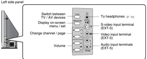
Connecting terminals on the back of the TV → "Connecting External devices" (P. 10)
