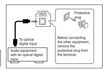
Connect an optical digital cord (not supplied) between the optical digital input terminal on the other equipment and the CD OPTICAL DIGITAL OUTPUT terminal.
