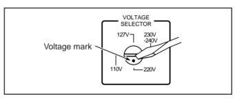
Use a screwdriver to rotate the voltage selector so the voltage number the voltage mark is pointing at is the same as the voltage where you are plugging in the unit. (See the back cover page.)
