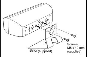
You can install the front and center surround speakers on the wall. When installing the front speakers on the wall, do not attach the stands.
