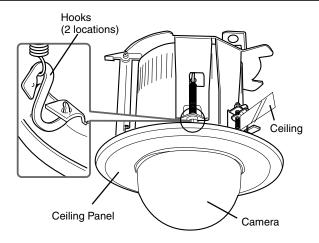
Attach the ceiling panel (supplied) to the 2 hooks on the Ceiling Recessed Bracket.
