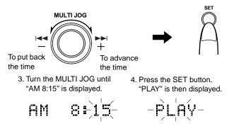
When "Play" is displayed, it is necessary to set the Timer Play or Timer Recording function.
