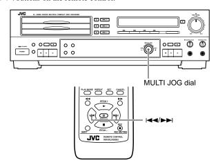
When the last track on a CD loaded in the 3-CD changer is advanced to the next track, playback moves to the first track on the next CD. There is no effect when the last track on the CD loaded in the CDR is advanced.
