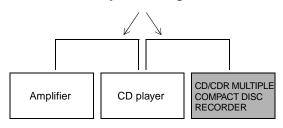
The COMPU LINK functions provided with JVC products come in the form of COMPU LINK-4, COMPU LINK-3 or COMPU LINK-1. They are compatible, and the difference between them is that COMPU LINK-3 has the functions of COMPU LINK-1 with some additional functions as well.
