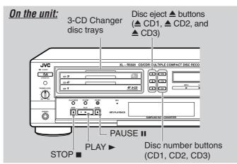
**1** Load discs onto the 3-CD Changer disc trays (see the left).
