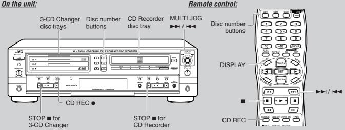
1 Load discs onto the 3-CD Changer disc trays and a recordable CD-R or CD-RW onto the CD Recorder disc tray.
