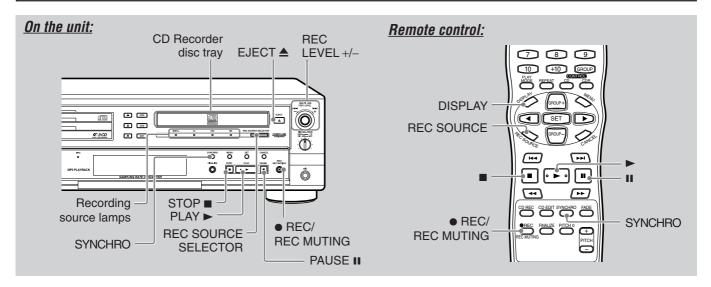
1 Load a recordable CD-R or CD-RW onto the CD Recorder disc tray.
