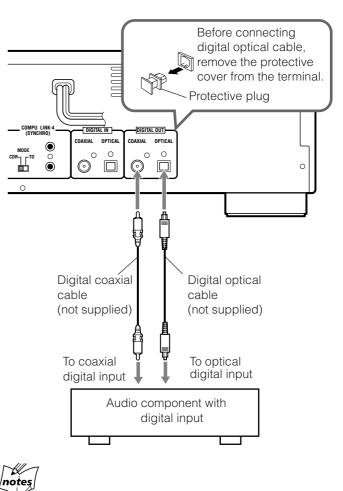
When this unit cannot recognize a component connected to the DIGITAL IN COAXIAL or OPTICAL terminal, "UNLOCK" appears on the display. If this happens, press PLAY ► for 3-CD Changer so that the connected component will be recognized.
