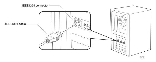
When connecting the IEEE1394 cable from camera recorder to other IEEE1394 device such as PC, make sure the following instructions, otherwise the IEEE1394 circuit device may be destroyed.
