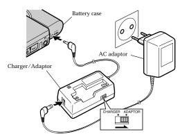
The unit is in the standby condition when the AC adaptor and charger/adaptor are connected. The primary circuit is always "live" as long as the AC adaptor is connected to an electrical outlet.
