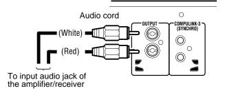
If you are connecting the unit to a JVC audio component and using the CompuLink-3 remote control system, connect the units with the accessory CompuLink cord. Either one of the COMPULINK-3 (SYNCHRO) ports in the back of this unit can be used.
