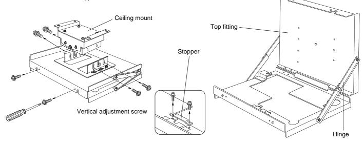
Use care to prevent the top fitting from dropping during the installation work since this could result in injury or damage.
