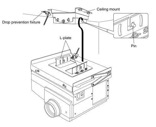
**2** Fasten temporarily with the vertical angle adjustment screws (4) which were removed. After fastening with the vertical adjustment angle screws (4), perform the adjustments described on page 13.
