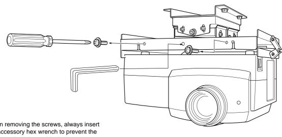
When removing the screws, always insert the accessory hex wrench to prevent the projector dropping suddenly.
