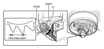
7 Tighten the fastening screw of the focus adjustment ring Hold and press the focus adjust gear between your fingers in the direction of the arrows in the diagram, and tighten the fastening screw of the focus adjustment ring.
