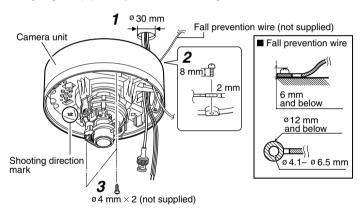
Note The screws for mounting the camera are not provided. Use a suitable type of screws according to the material of the mounting location.
