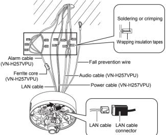
Connect the AC 24 V power cable, alarm cable, and audio cable to their respective connectors by crimping them or soldering them. Wrap unused connectors and the ends of unused cables with insulation tape and waterproof tape.
