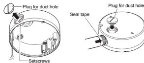
\* This illustration does not show the inside of the camera body for convenience of explanation. \*Place the duct hole plug that you removed into the duct hole at the bottom of the camera.
