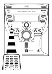
When using the remote control, point it at the remote sensor on the front panel.
