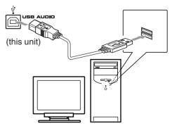
• Use "USB series A plug to B plug" cable when connecting.
