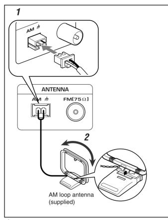
**1** Connect the AM antenna to the AM terminal on the rear of the unit.
