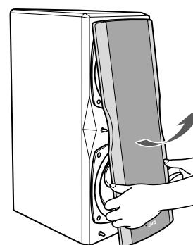
To attach the speaker grille, put the projections of the speaker into the holes of the speaker grille.
