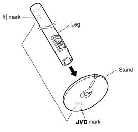
**3** Fix the leg to the stand with three of the supplied screws (long: M4 x 25 mm).
