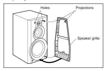
To remove the speaker grille, inserting your fingers at the top of the speaker grille, pull towards you. Then pull the bottom towards you.
