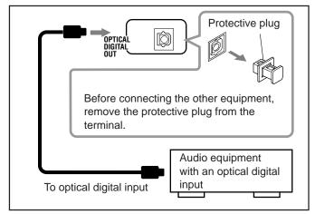
Connect an optical digital cord (not supplied) between the optical digital input terminal on the other equipment and the OPTICAL DIGITAL OUT terminal.
