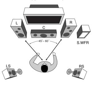
After connecting the speakers, set the speaker installation information properly. You can use Quick Speaker Setup for it (see page 18).
