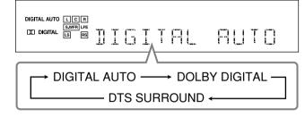
When "DOLBY DIGITAL" or "DTS SURROUND" is selected, the DIGITAL AUTO indicator goes off, and the corresponding digital signal format indicator lights up on the display.
