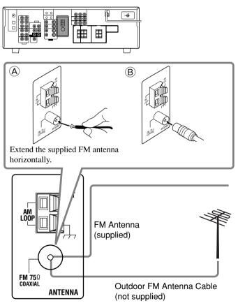
Connect the supplied FM antenna as temporary measure to the FM 75  $\Omega$  COAXIAL terminal—(A)
