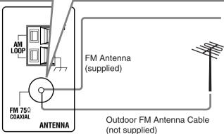
Connect the supplied FM antenna as temporary measure to the FM 75  $\Omega$  COAXIAL terminal— $\widehat{\mathbb{A}}$
