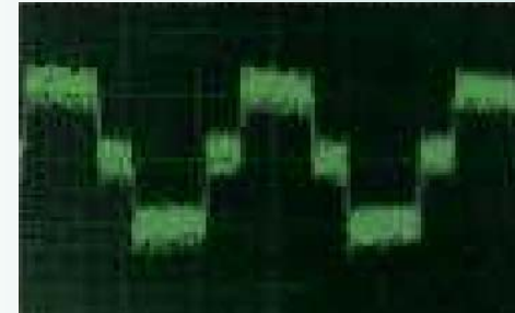
-90dB, 1kHz Sine Wave: Bit Expansion Off
