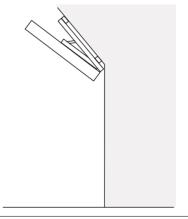
■ Do not install the Wall Mounting Unit on a non-vertical wall.
