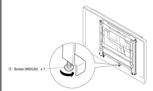
\* Check to make sure that the lever is securely fastened and the plasma display does not rattle.
