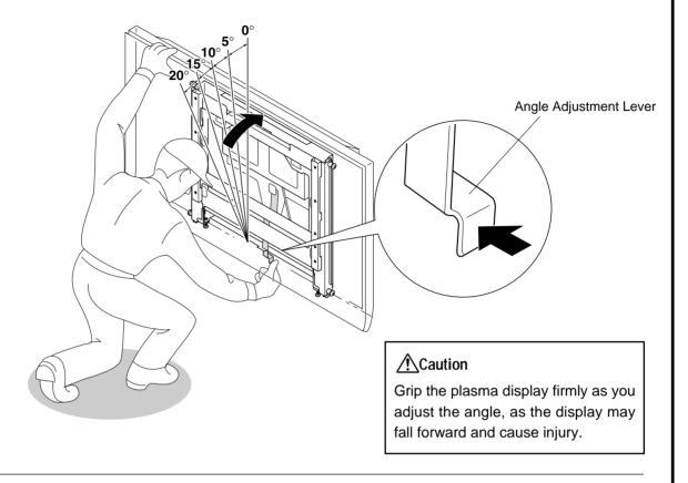
8. Fasten the Angle Adjustment Lever.
