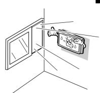
■ Do not install the unit in a location exposed to direct sunlight or strong light, as viewing the plasma display in an overly bright environment can be tiring for the eyes.
