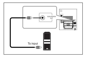
Connect the input jack of a powered subwoofer to the SUB WOOFER OUT jack, using a monaural audio cord (not supplied).
