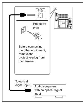
Connect an optical digital cord (not supplied) between the optical digital input terminal on the other equipment and the CD OPTICAL DIGITAL OUTPUT terminal.
