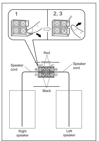
**1** Press and hold the clamp of the speaker terminal on the rear of the unit.
