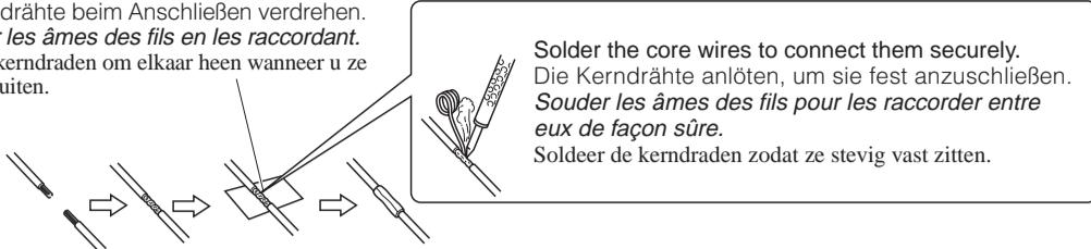
Solder the core wires to connect them securely.
