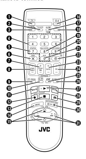
Buttons with a small dot on the left side of the name can also be used to operate your JVC TV while holding down the **TV** button. (IF "Operating JVC TVs" in the right column)
