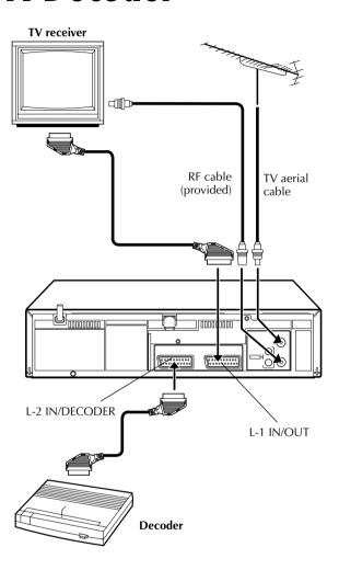
The L-2 IN/DECODER connector can be used as an input connector for an external decoder (descrambler). Simply connect a decoder and you can enjoy the variety of programming that is available through scrambled channels.
