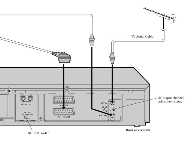
The video recorder sends picture and sound signals via the RF connecting cable to your TV on UHF channel 36.
