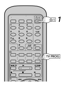
The Auto Set Up function sets the tuner channels, clock and Video Plus+ assigned Guide Program numbers automatically when the 0/1 button on the recorder/remote is first pressed to power on the recorder after you plug the mains power cord into a mains outlet.
