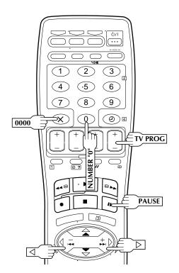
Insert editing replaces part of the recorded scene with new material. Both the picture and Hi-Fi audio soundtrack are replaced with new ones, while the normal audio soundtrack remains unchanged. If you wish to change the normal audio track as well, use the audio dubbing function simultaneously. Use your video recorder as the recorder.
