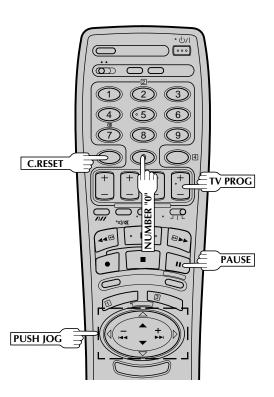
Insert editing replaces part of the recorded scene with new material. Both the picture and Hi-Fi audio soundtrack are replaced with new ones, while the normal audio soundtrack remains unchanged. If you wish to change the normal audio track as well, use the audio dubbing function simultaneously. Use your video recorder as the recorder.
