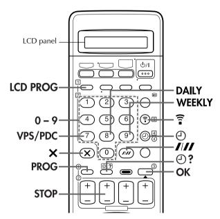
With the SHOWVIEW system, timer programming is greatly simplified because each TV programme has a corresponding code number which your recorder is able to recognize. You can use the remote control with LCD panel to enter the SHOWVIEW number.
