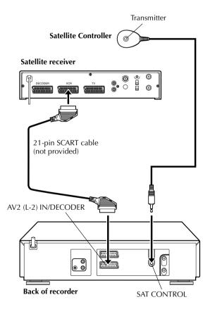
The following procedure is required if you receive satellite channels through a satellite receiver. Approximately 20 seconds before the SHOWVIEW timer programming ( pg. 26) or Express timer programming ( pg. 28) starts, the recorder sets its input mode to "L-2" and automatically switches the satellite receiver's channels using the provided Satellite Controller.
