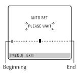
When you have connected the video recorder to a TV offering T-V Link via a fully-wired 21-pin SCART cable ( pp. 9) and the TV is turned on, the recorder automatically performs the Preset Download ( pp. 12) even if you select "Auto" for Auto Set Up function.
