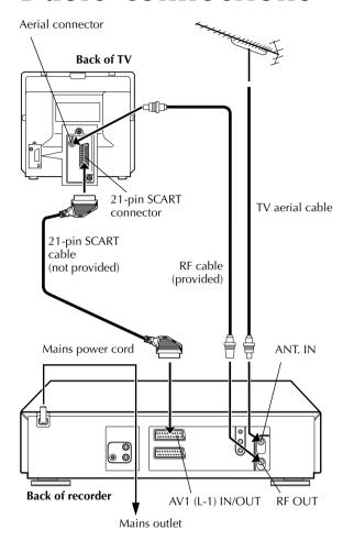
Make AV connection if your TV has a 21-pin AV input connector (SCART) in order to reduce the possibility of interference. With AV connection, you can enjoy stereo playback of video tapes if you are using a stereo TV.
