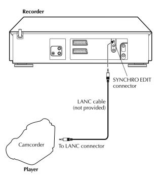
The Synchro Editing function synchronizes the start of the playback and recording operations when starting an edit operation using a camcorder with LANC connector and your recorder.
