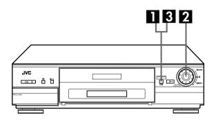
You can programme a timer recording that starts within 24 hours using the JOG dial on the recorder.
