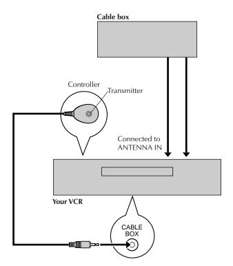
This procedure is required if you receive your TV channels through a cable box (descrambler). The Controller allows the VCR to automatically switch the cable box channel during timer-recording. The Controller is effective for recording shows that have been programmed using VCR Plus+ (F pg. 43) or Express Timer Programming (F) pg. 47).
