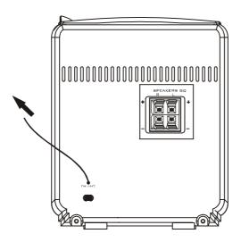
**AM**: The AM bar antenna is inside the cabinet of the main unit. You may need to change the position of the main unit until you find the position that provides the best reception for your favorite AM stations.
