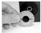
With the disc removed, a different disc can be inserted to change the angular spacing. The 14 position detent disc (included with your bracket) is for use with the optional Fujifilm 0.8X wide angle lens (available from Fujifilm for the Fuji MX-2900 camera).
