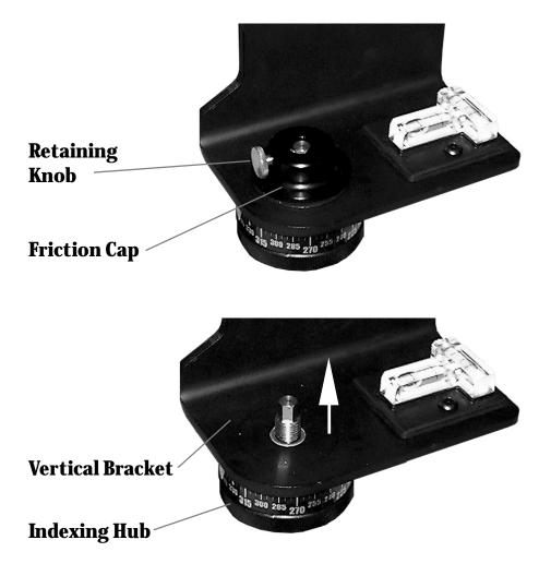
Once the Friction Cap has been removed, separate the Vertical Bracket from the Indexing Hub. You might need to wiggle the pieces as you pull them apart.
