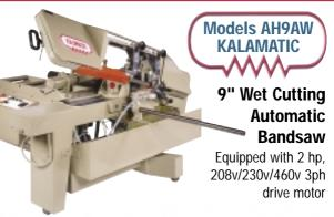
Operators can set-up the Kalamatic quickly and the procedure is easily learned. The feed roller and saw head is lifted, stock loaded and positioned, stock stop adjusted for proper length, the number of pieces required is entered in the counter and then the cutting cycle is initiated by the operator. After that, the saw operates automatically until all pieces are cut or the stock is exhausted.
