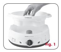
Pour sufficient clean, tap water, up to 1 litre, into the water reservoir of the steamer base and ensure the maximum 'MAX' level on the water window is not exceeded. If cooking for long periods of time ensure the water level does not fall below the minimum 'MIN' mark. During operation, extra water can be poured into the water reservoir through the easy to fill water spouts at either end of the liquid collection tray.
