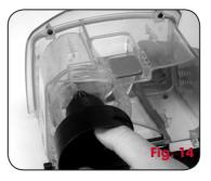
Press the `PUSH' button located beneath the hose inlet connection on the front of the dust container. The bottom of the container will release. Grip the two pockets at the base of the cone with two fingers, twist anticlockwise to `OPEN' and pull to remove the cone.
