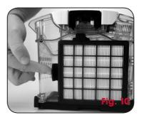
Shake and tap the HEPA filter until all the fine dust particles are removed. After approximately 6 months the HEPA filter should be replaced. This period is dependant upon the frequency of use and type of dirt being subjected to the vacuum. The HEPA filter can also be hand washed in warm water.
